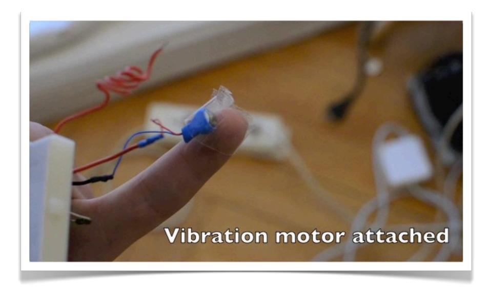
» Arduino based electromagnetic field sensor» Vibration motor gives haptic feedback
