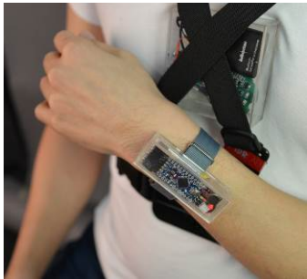
Figure 1. WearBEAT chest mount and bracelet wearable state
