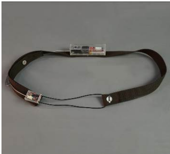
Figure 5. WearBREATH breathing input belt
