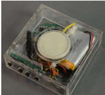
Figure 2. WearBEAT body-sound input chest mount unit
