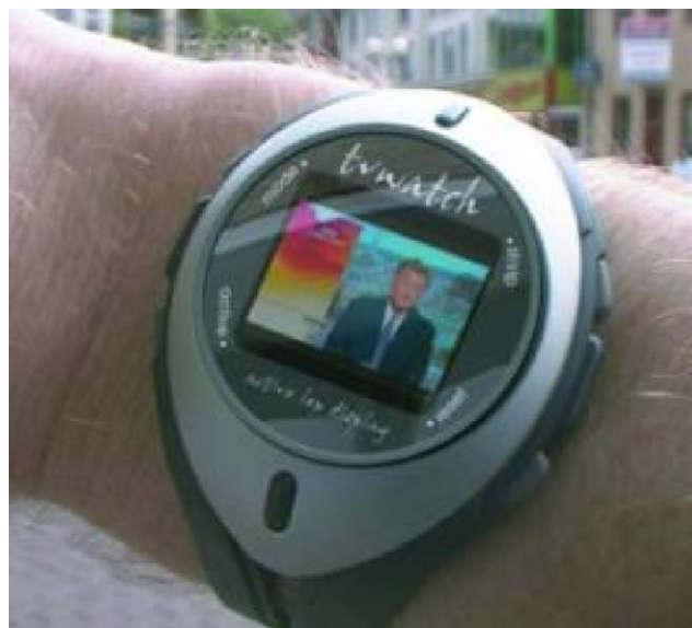
Fig. 15. Wrist watch with OLED display (adapted from [56]).
