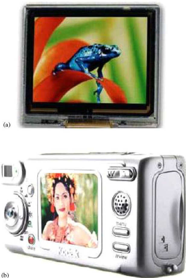
Fig. 12. (a) Kodak Nuvue Display AM550L. Characteristics: diagonal: 5.5 cm, weight: 8 g, peak luminance: 120 \text{ cd/m}^2 , power consumption: 400 mW. (b) Kodak EasyShare LS633 zoom digital camera equipped with the AM550L display (adapted from [73]).
